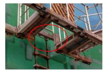
**Figure 1:** Pilot ladder/trapdoor showing the non-compliant horizontal cross-member.
